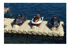
Our **Multi Port** consists of **modular floating cubes** 50 x 50 x 40cm and **body parts** 100 x 100cm equipped with **horizontal** and **side rollers**. The entry part is V-shaped with a 1st roller at water level. The **raised-bow head part** welcomes the bow of your jet ski.
